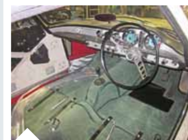
October 2012 Interior The interior is unique to Jensen-built cars so spares are ultra-rare. Most components had to be painstakingly remade by a specialist.
