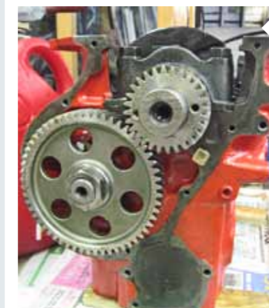
2007-2011 Engine work Engine has to be rebored to 2.0-litre. Mods include steel timing gears and a high-lift cam.
